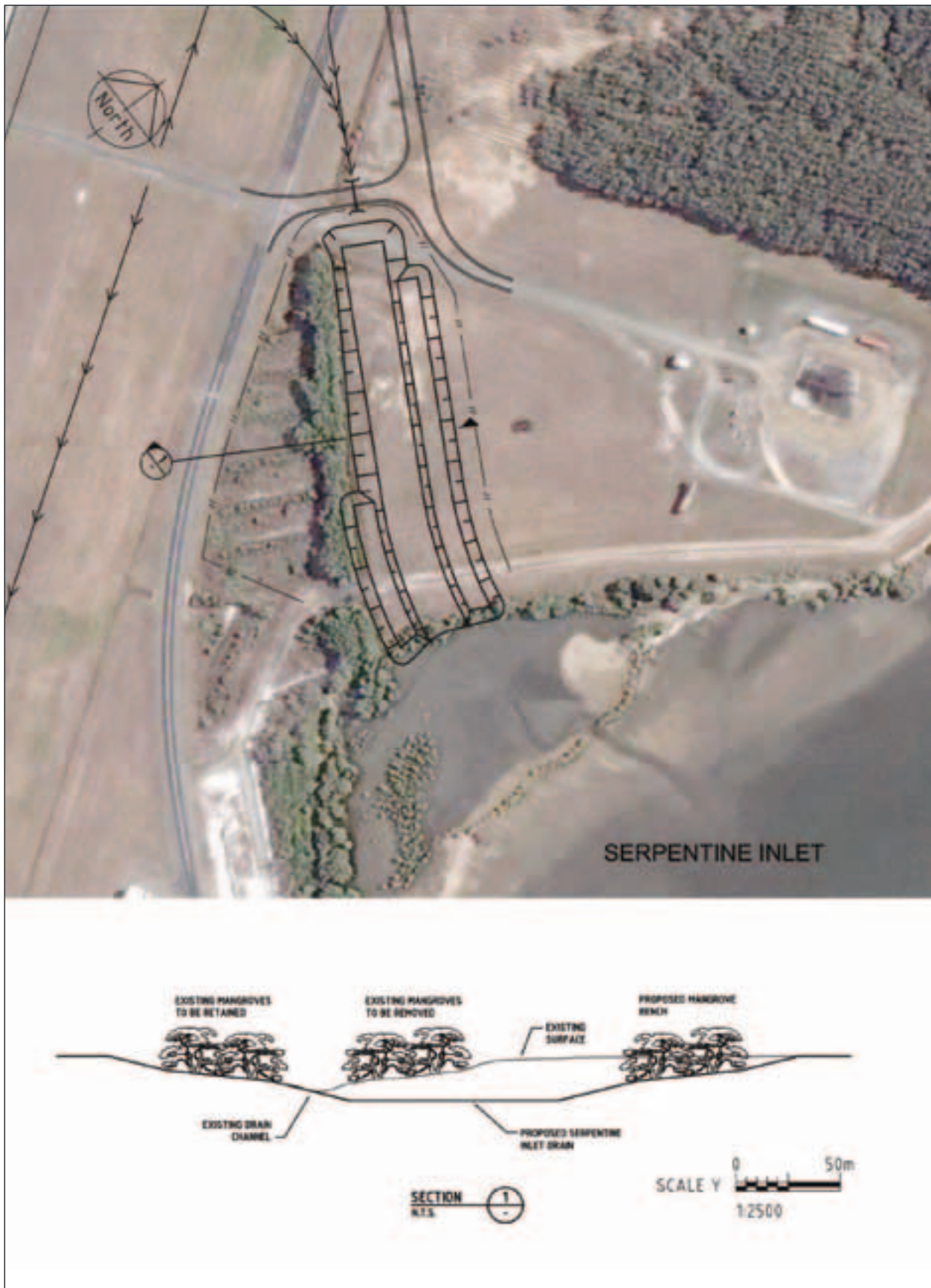
Figure 7.3c: Serpentine Inlet Drain (Existing and Proposed).
